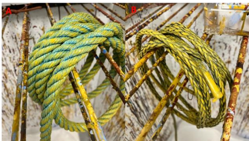
Figure 14: Examples of unsuccessfully coated polyolefin2 (A) and recycled polyolefin2 (B) with standard coating.
