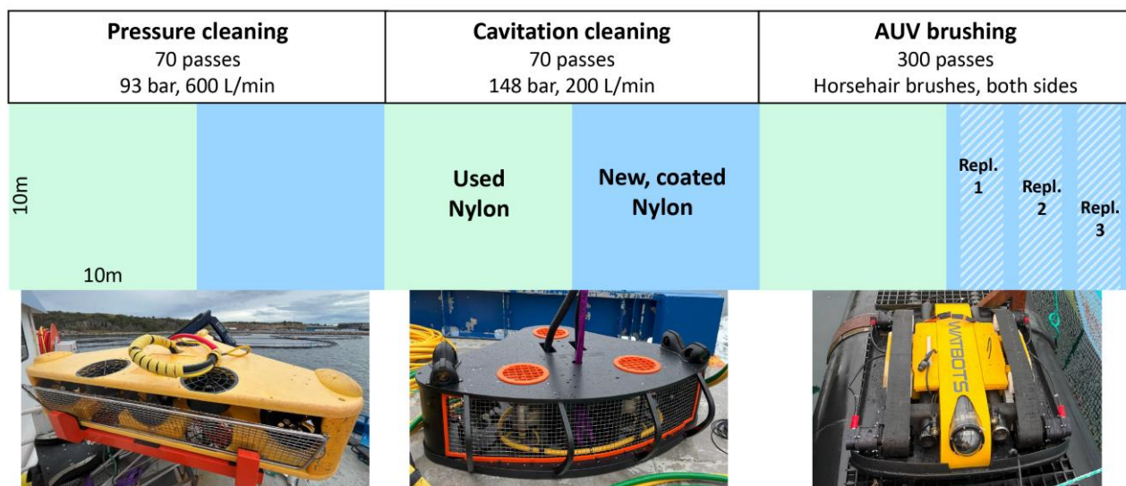
Figure 7: Schematised experimental set-up to simulate 10 months of net cleaning at sea testing three technologies on two net materials.
