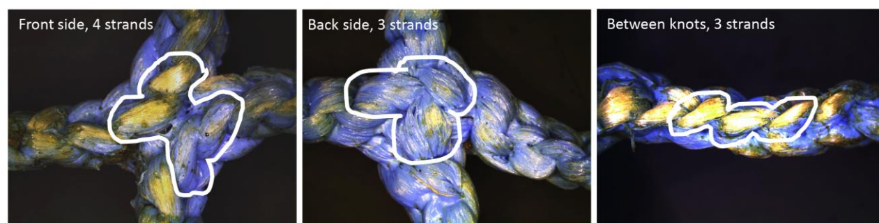
Figure 9: Net strands chosen for assessment of coating integrity located on front and back side of the knot, as well as between knots.
