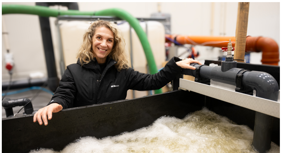
Siri Tømmerås from AKVA group stands by the mini-CO 2 degasser, which is used to test how factors such as alkalinity, pH, salinity and temperature affect degassing efficiency. Photo: AKVA group
